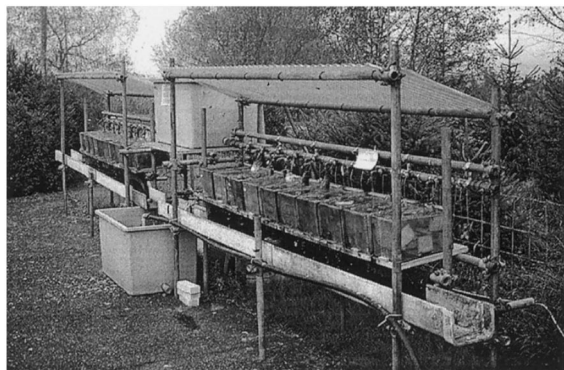
Fig. 1. The flow-through aquaria system used for periphyton colonization and long-term copper exposure.
